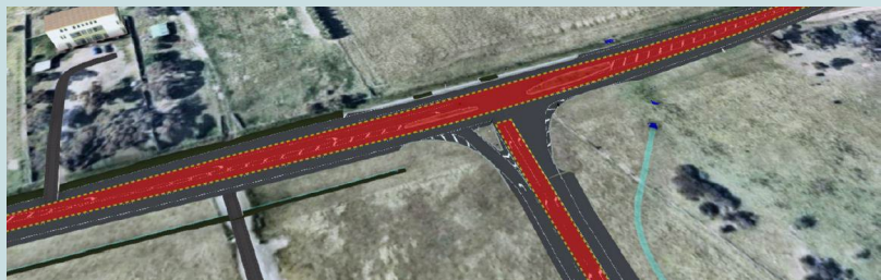
Stage 3: Traffic lanes will be divided, with a central work zone established
