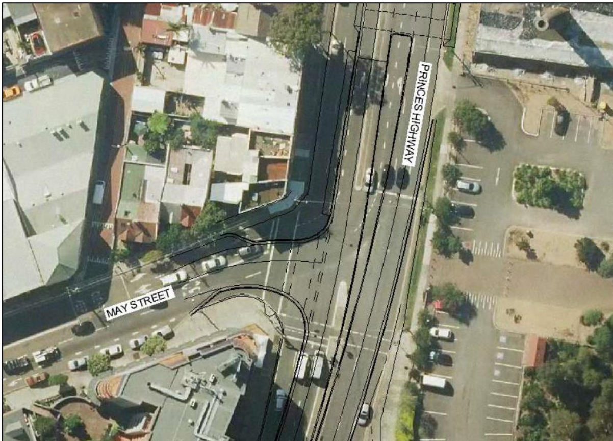
Figure 1: May Street and Princes Highway new intersection arrangement.
