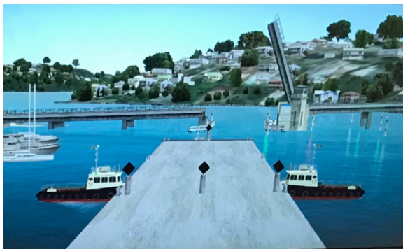
1. Transport of steel shell unit through Spit Bridge.
