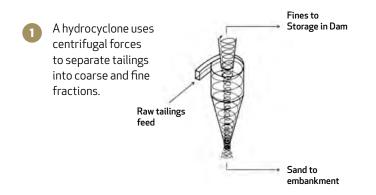
Once separated, the coarse sand (hydrocyclone underflow) is delivered to, and hydraulically deposited into cells on the embankment for compaction.
