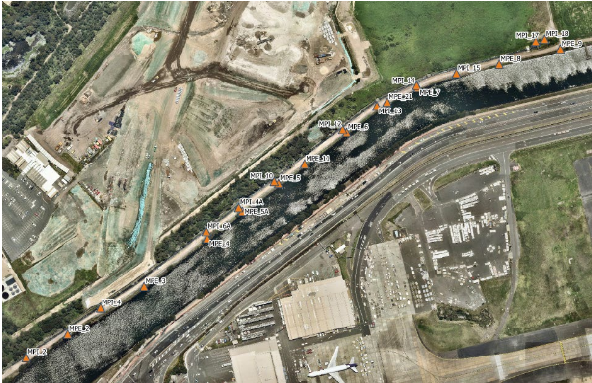
Figure 1, Leachate monitoring well sampling locations.
