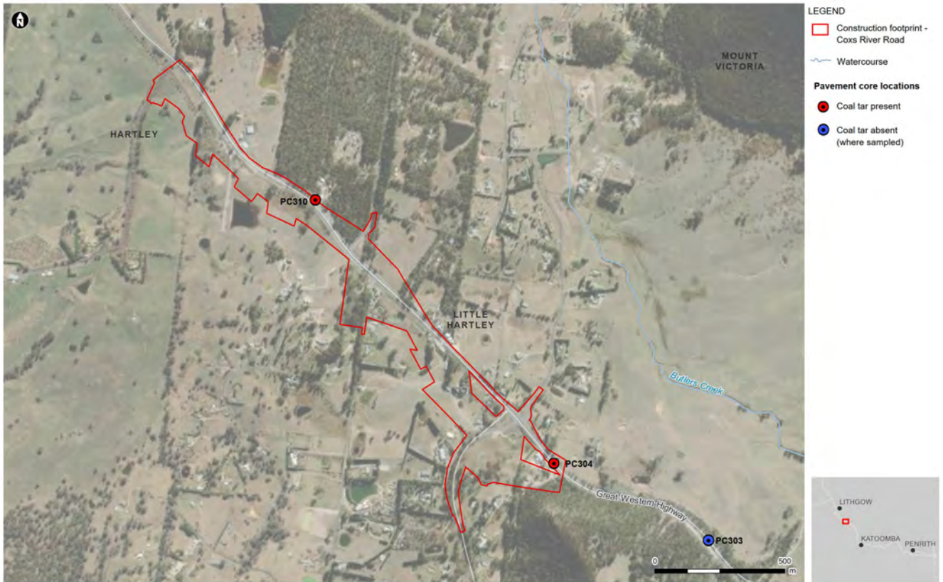
Figure 1.2: Pavement core locations for CRR study area
