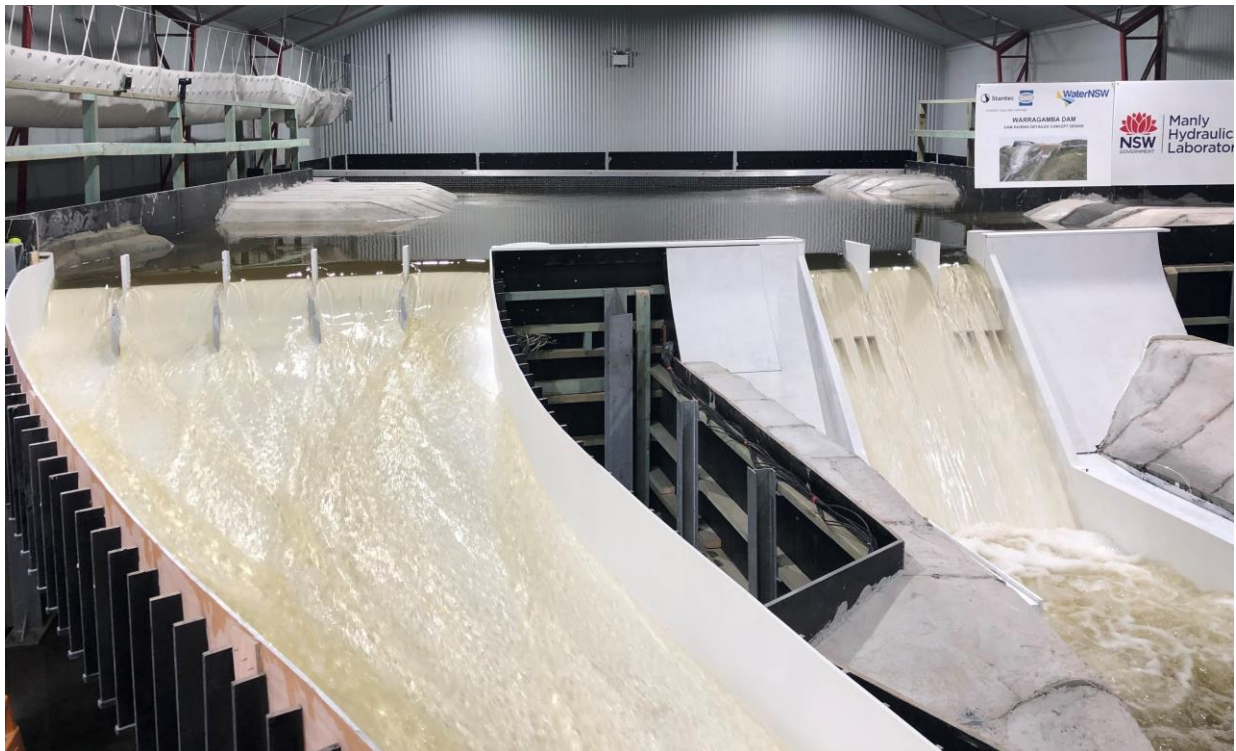
Figure 10. Image of the scale physical hydraulic model
