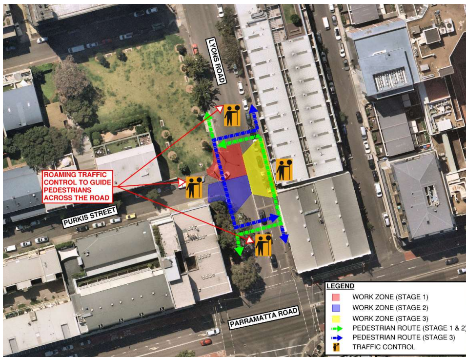
Figure 4: Traffic and Pedestrian Management Strategy – Lyons Road, at the intersection with Purkis Street
