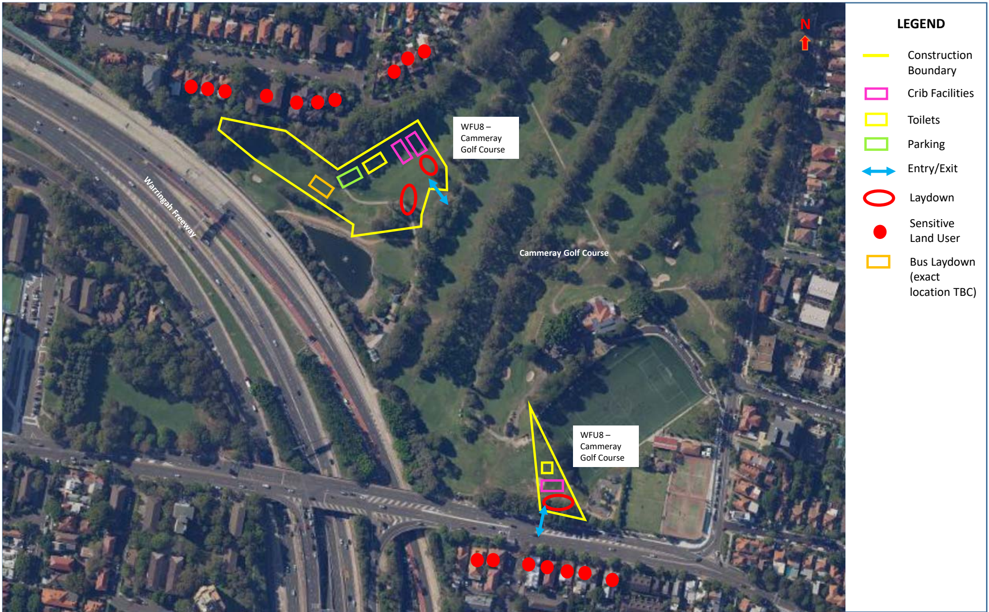
Indicative Site Layout: WFU8 – Cammeray Golf Course Western Harbour Tunnel and Warringah Freeway Upgrade SSI-8863 Stage 2 – Warringah Freeway Upgrade
