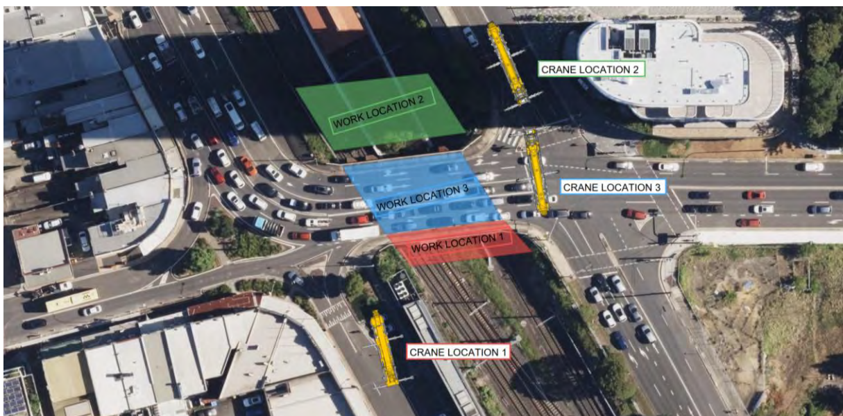
Figure 6-2 Temporary crane locations and work locations
