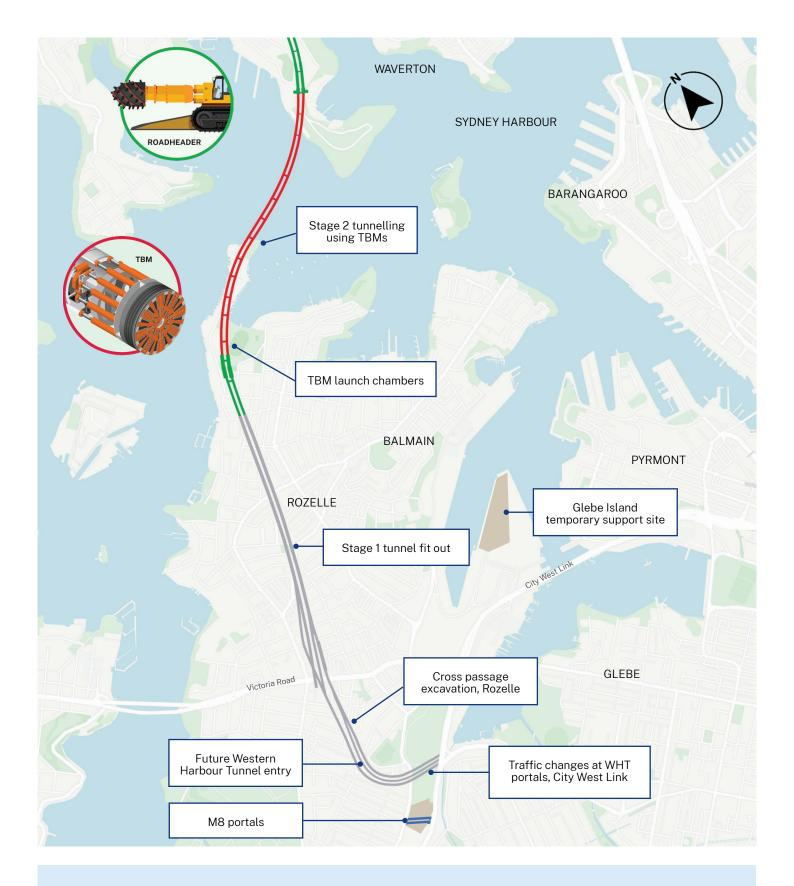
Work is underway this year to create a direct connection to Sydney's motorway network via the M8 tunnels below Rozelle. This connection is a vital step in efficiently managing construction logistics and enabling our trucks to access the tunnels without relying on surface roads.
