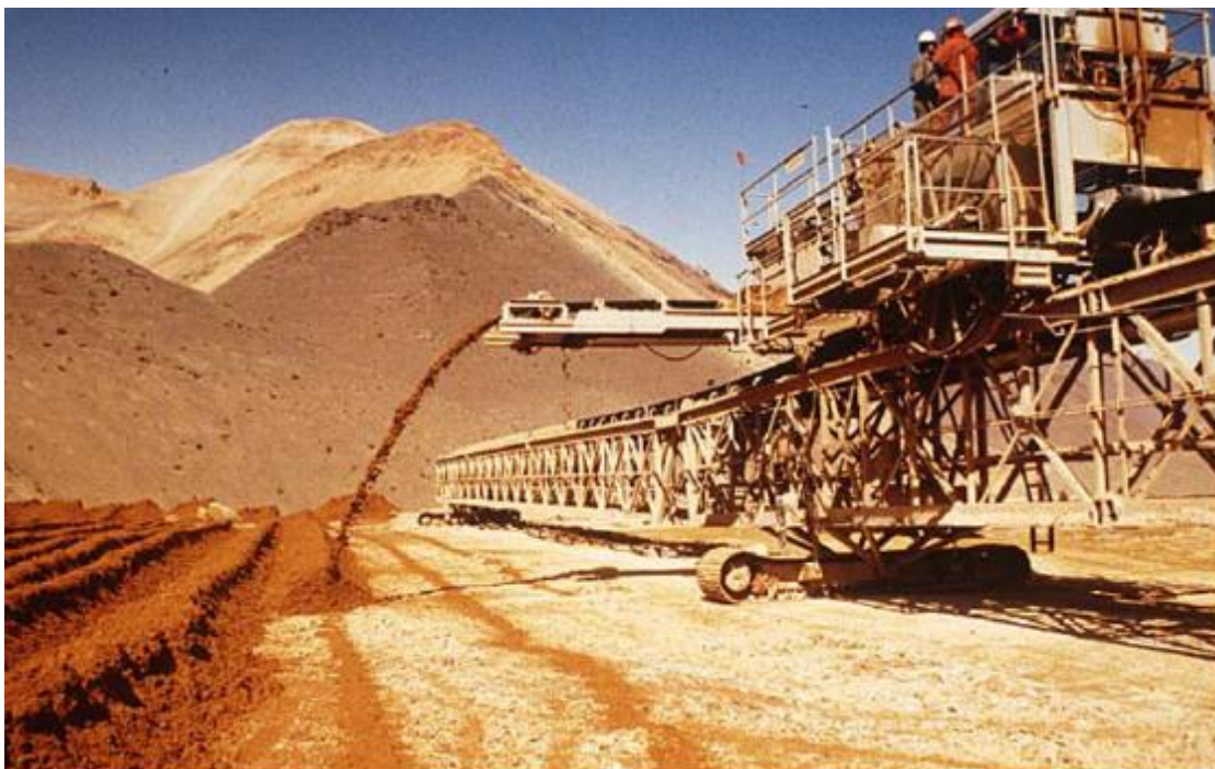
Figure 5.2 Dry stack tailings deposition at La Copa Mine, Chile
