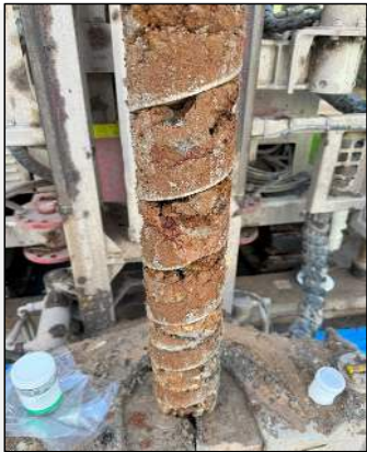
Photo 10: 16/01/2024: Representative image of soil material (BH155)
