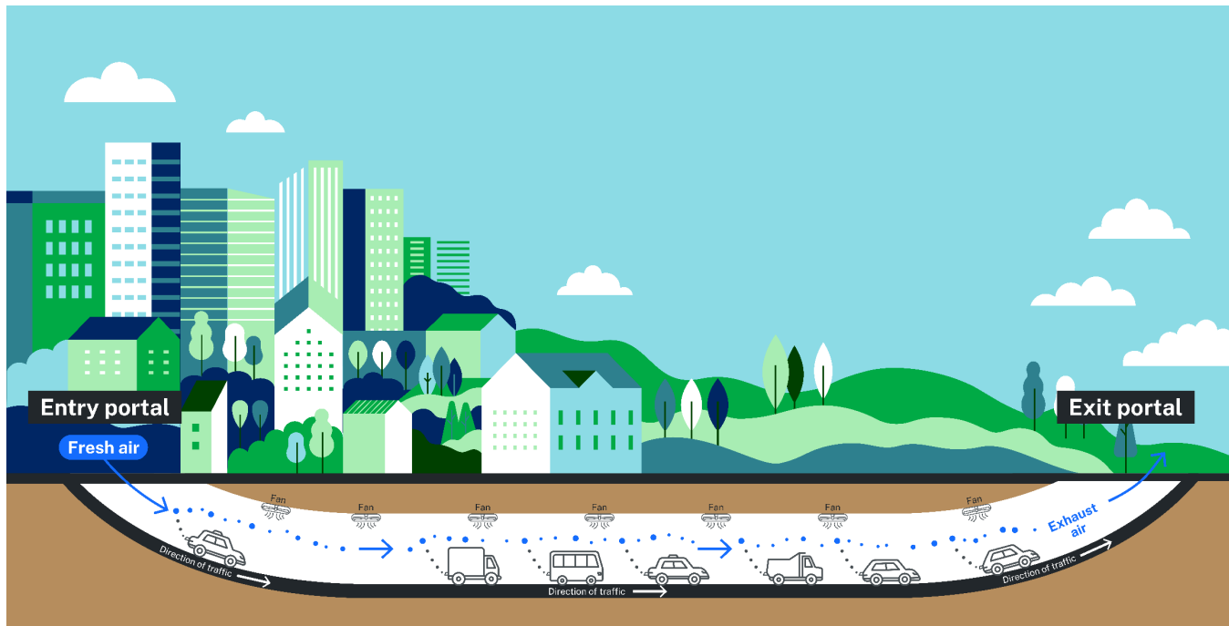
Figure 1: Tunnel ventilation through portals
