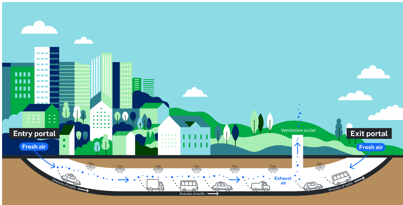
Figure 2: Tunnel ventilation through ventilation outlets
