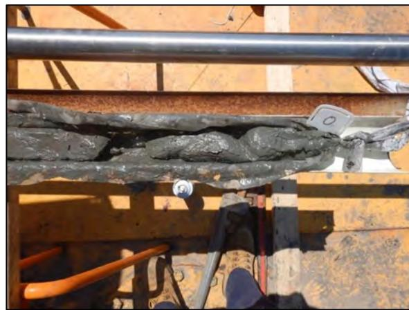
Fig. B 4      Site CBH4 sediment core, bottom to surface (left to right)
