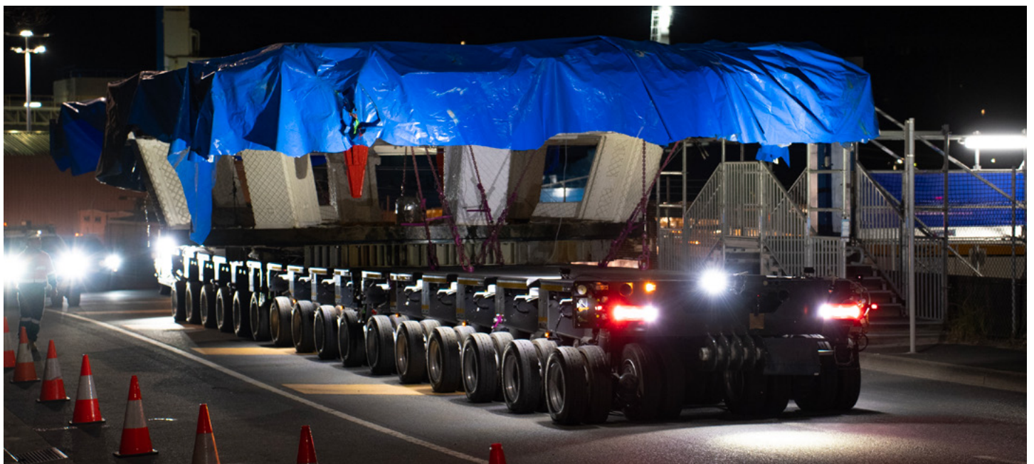
The first TBM part being delivered from Glebe Island across City West Link and into the WHT portals.
