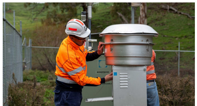
Figure 1: A Tapered Element Oscillating Microbalance (TEOM).
