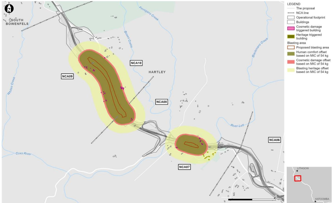
Figure 6-12 Buildings within the blasting minimum working distances
