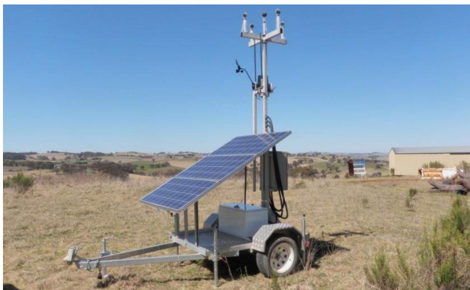
Plate 10-1: Quattrosound Directional Noise Monitor
