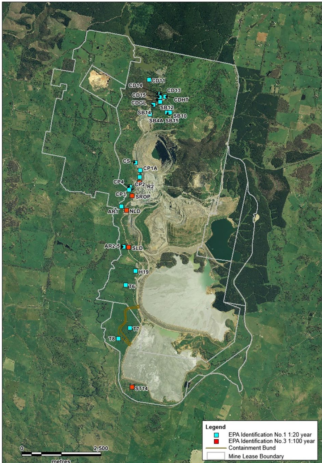
Figure 16-23 Sediment Control Structure Locations
