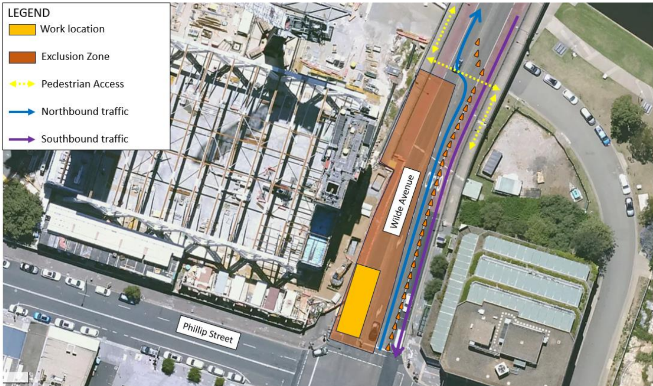
Image: Aerial view of work location, exclusion zone and traffic plan on Wilde Avenue.
