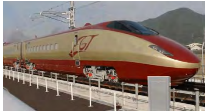
Kawasaki has developed an experimental Shinkansen train which can switch between standard and narrow gauges ii
