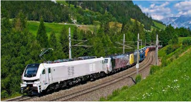
Stadler "Eurodual" Locomotive has 2800 KW using diesel, and up to 7,000 KW using electric power x
