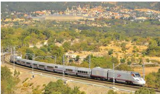
Talgo 250 Dual in Spain Note the supplementary diesel power behind the electric locomotive iv
