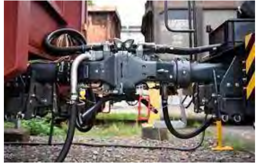
Digital Automatic Coupling systems are being developed in Europe, along with driverless shunting engines, to reduce terminal costs xi
