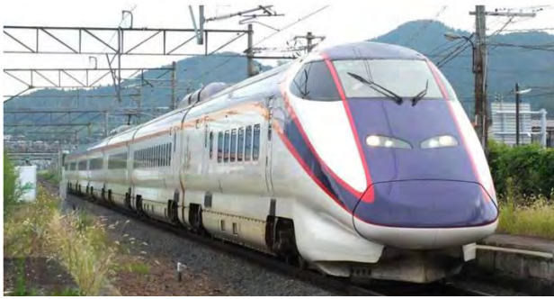
"Mini-Shinkansen" trains have a narrower loading gauge allowing services to extend to former narrow-gauge lines, although at lower speeds i
