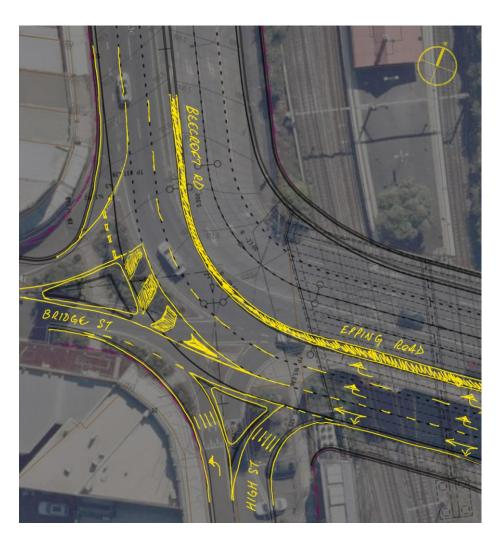
Figure 4-6 Alternate Northbound Lane Arrangement
