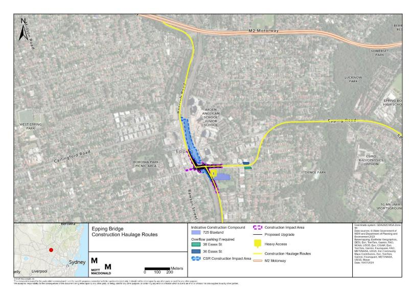
Figure 5-5 Construction haulage routes
