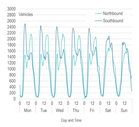
Figure 3-9 Hourly Vehicle Flow Profiles by direction (Oct, 2023)
