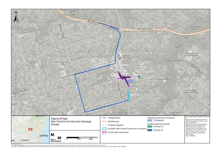
Figure 5-6 Rail corridor construction haulage routes
