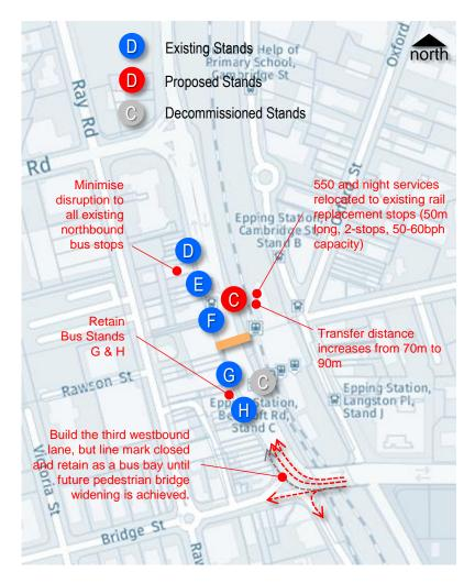
Figure 4-5 Alternate Northbound Bus Stop Arrangement
