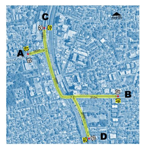
Figure 5-1 Extent of Construction Speed Zones
