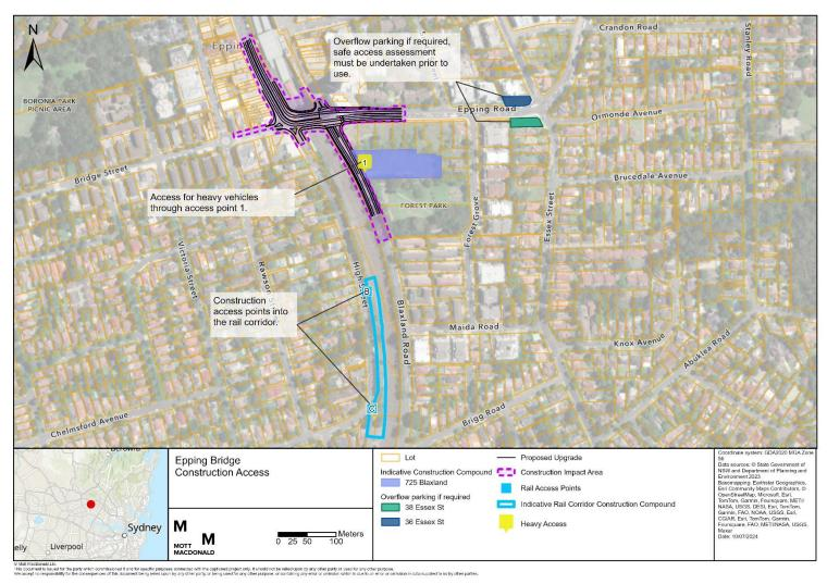
Figure 5-4 Construction site access and construction compound
