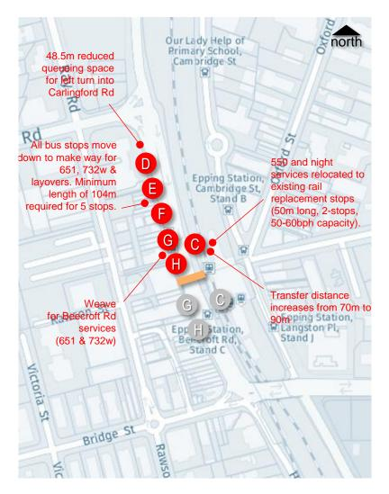
Figure 4-4 Revised Bus Interchange Configuration
