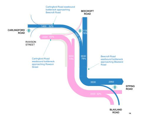
Figure 4-2 Existing Constrained AM Peak Capacity
