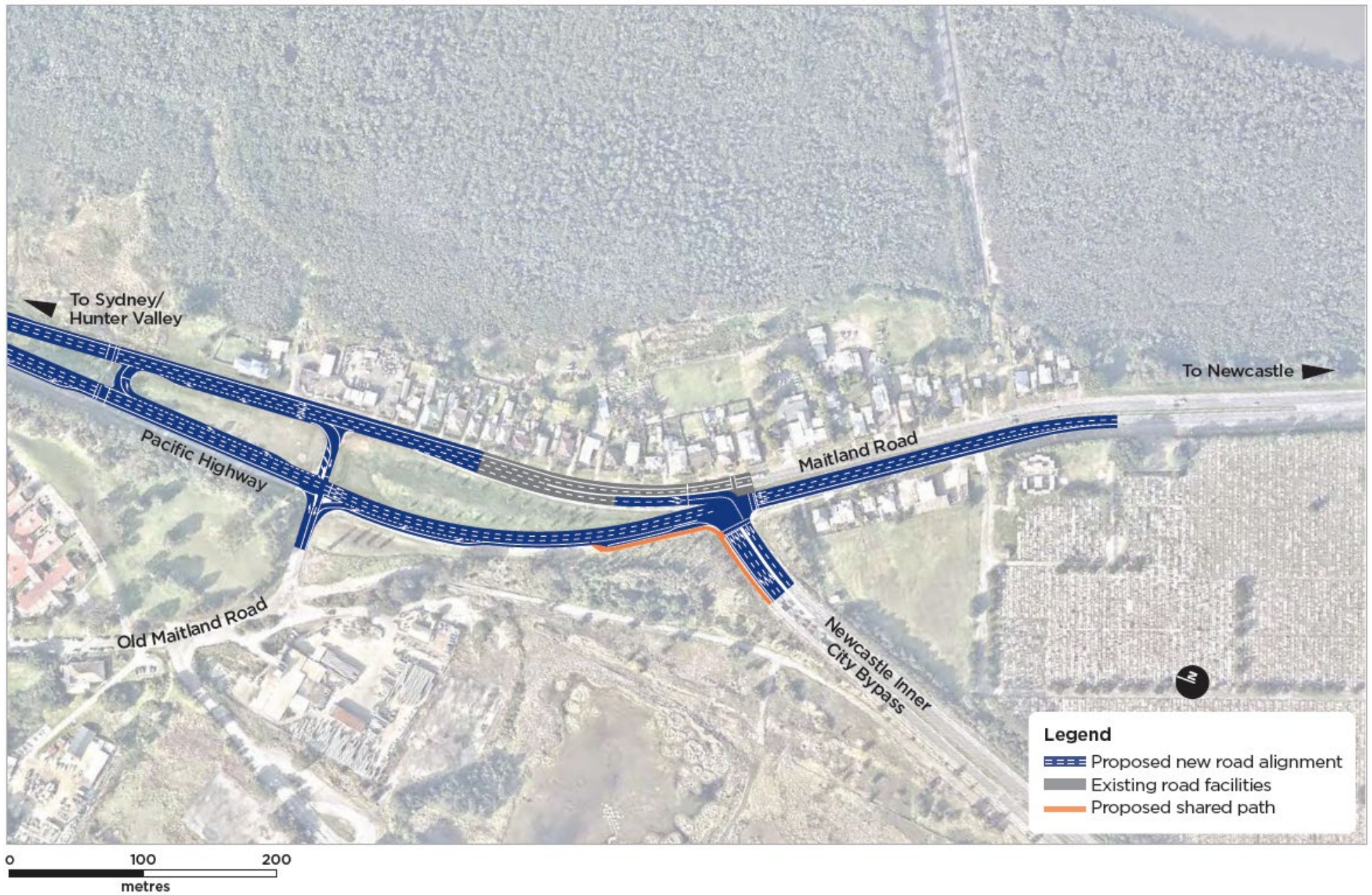
Figure 3.1f Hexham Straight Widening improvements
