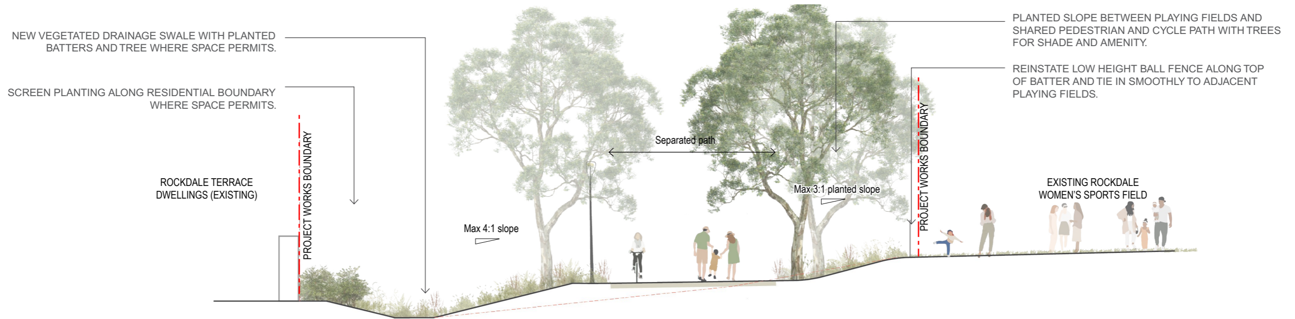
Figure 8-17: Section 02 - Typical section through ATC pedestrian and cycle path. Scale 1:100
