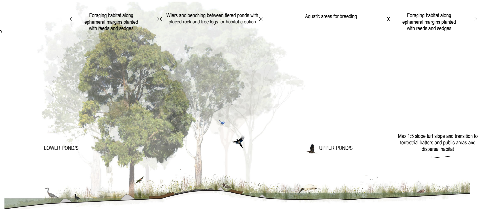
Figure 8-8: Typical section through tiered GGBF ponds
