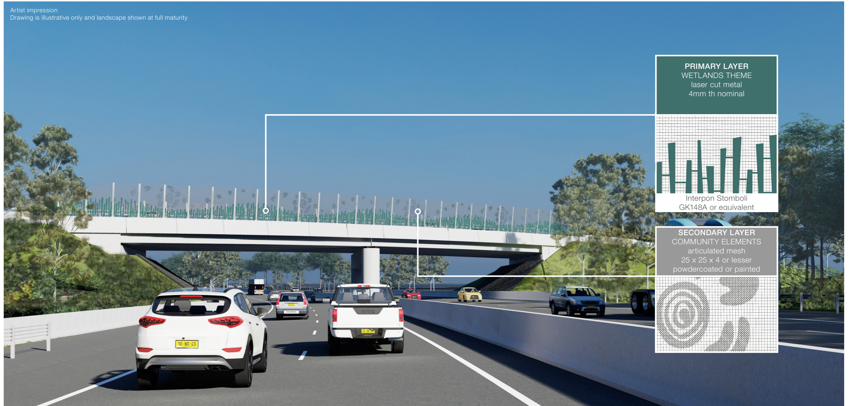
Figure 52: Safety screens - materials
