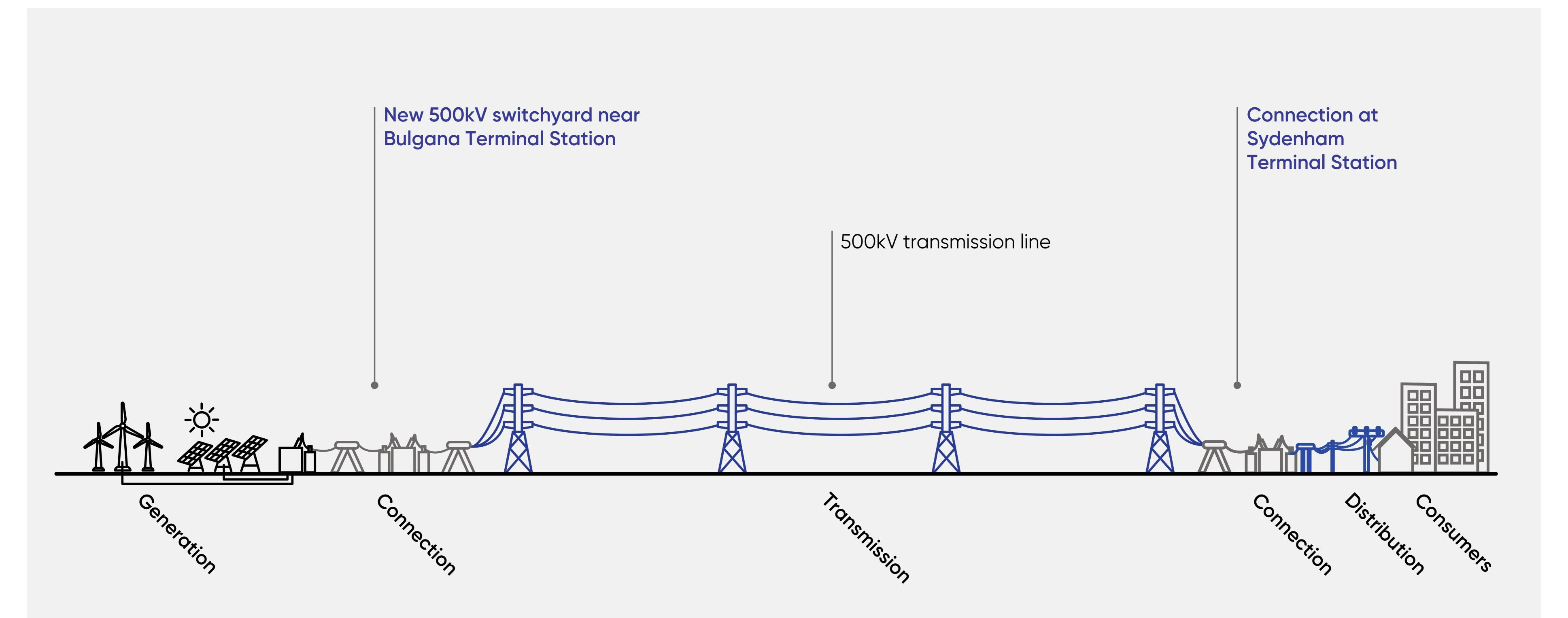
Proposed overhead 500kV double circuit transmission line from Bulgana to Sydenham
