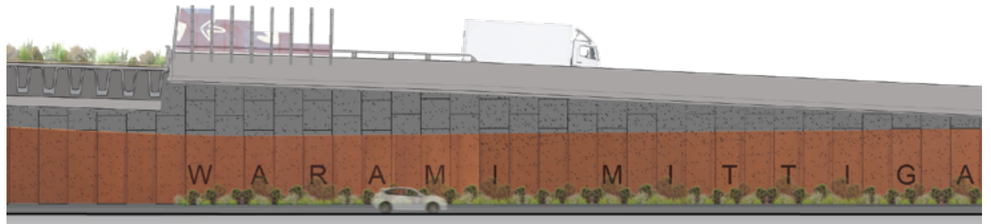
Figure 68. Pattern finish - Typical elevation - RSW wall
