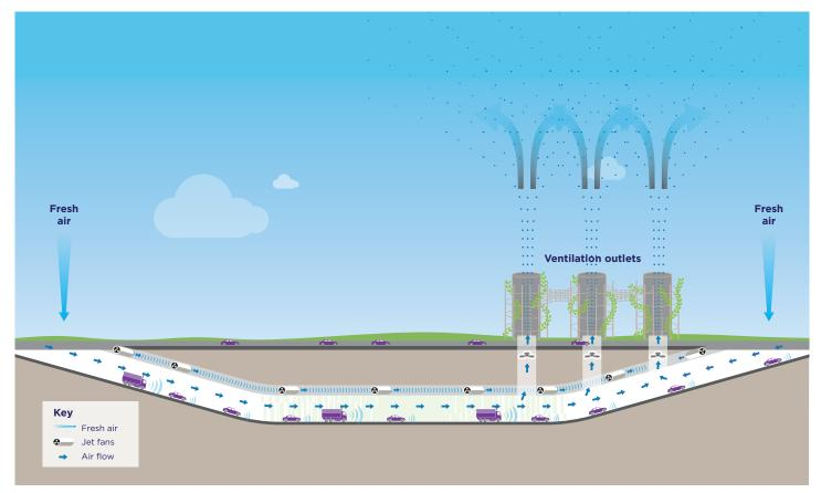
Modern tunnel ventilation ejects tunnel air high into the atmosphere
