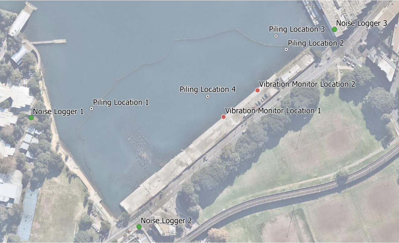
Figure C1 Vibration monitoring locations
