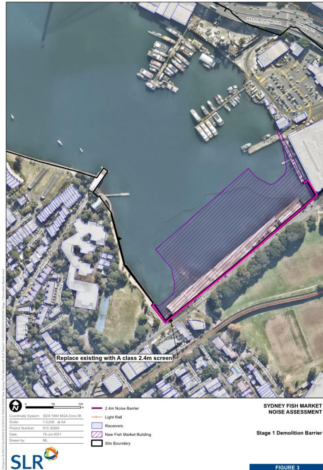
Figure 3 Stage 1 Demolition – 2.4m Hoarding Layout
