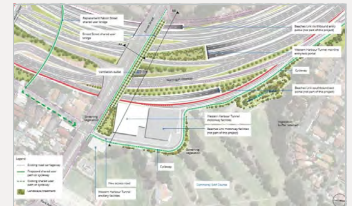
Figure B.3 Ernest Street Bridge Reference Design
