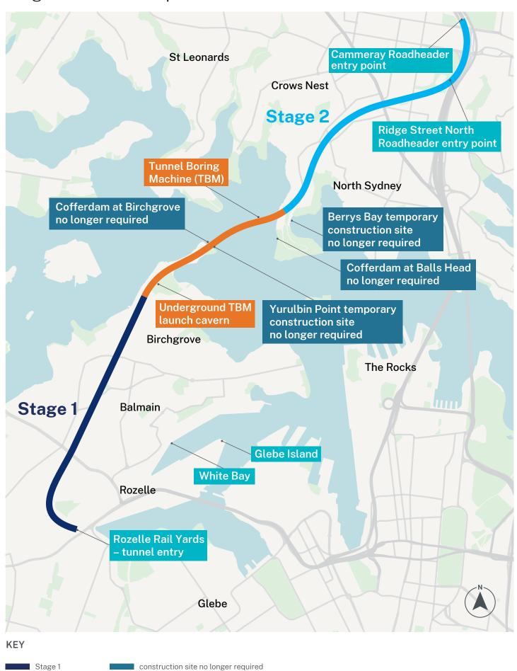
\* Stage 2 tunnel alignment is subject to detailed design and is not to scale
