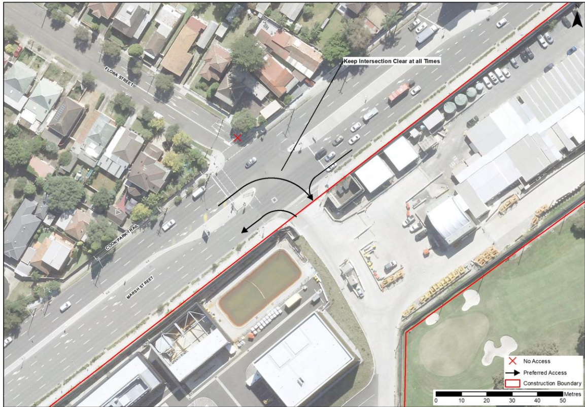
Figure 1 Access to C1 Arncliffe construction ancillary facility
