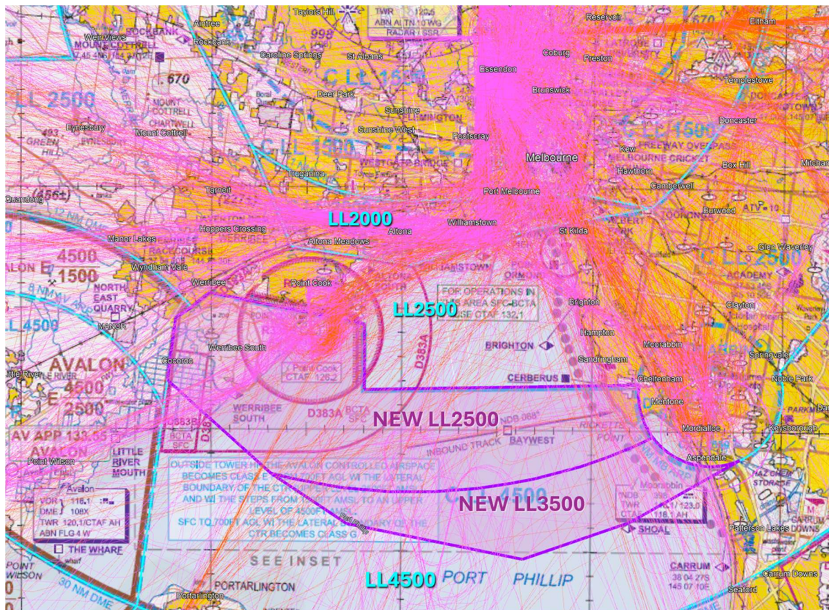
Figure 9: PHASE 1 - Historic aircraft tracks in Port Phillip Bay using the published VFR route - initial proposed airspace changes shown in purple.
