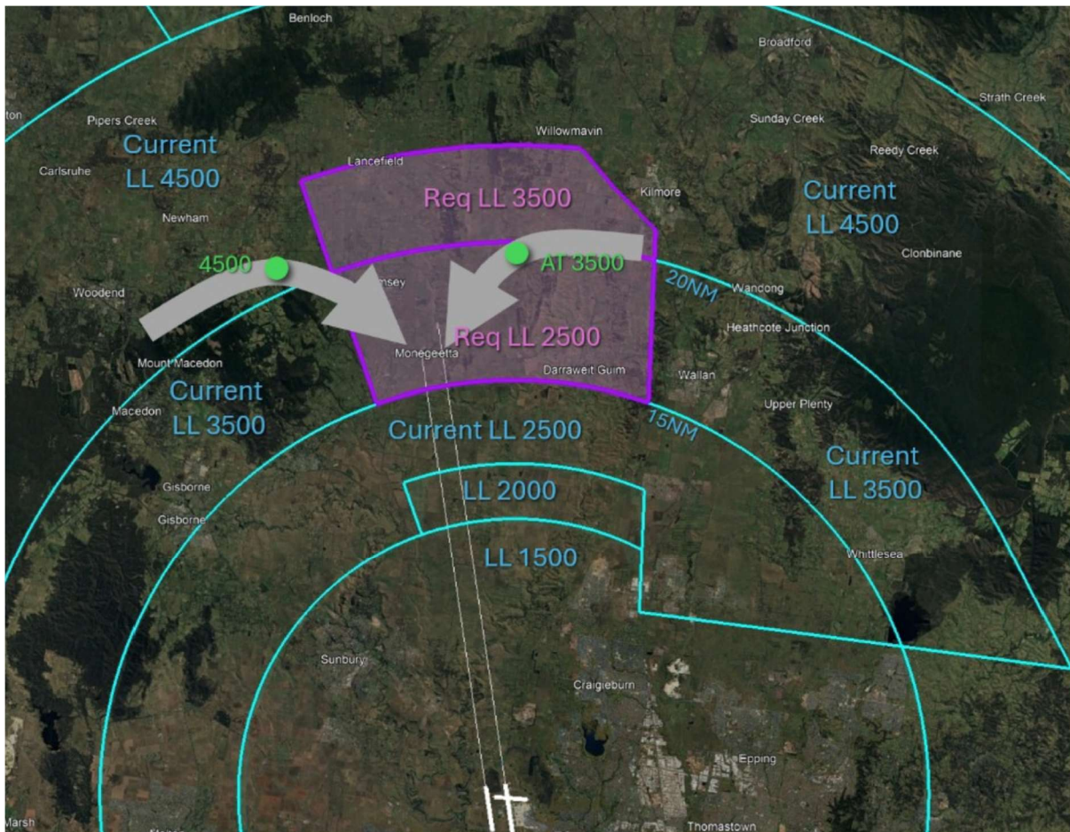
Figure 3: PHASE 1 – Initial proposed changes to control area steps to the north along with indicative aircraft altitudes for parallel arrivals
