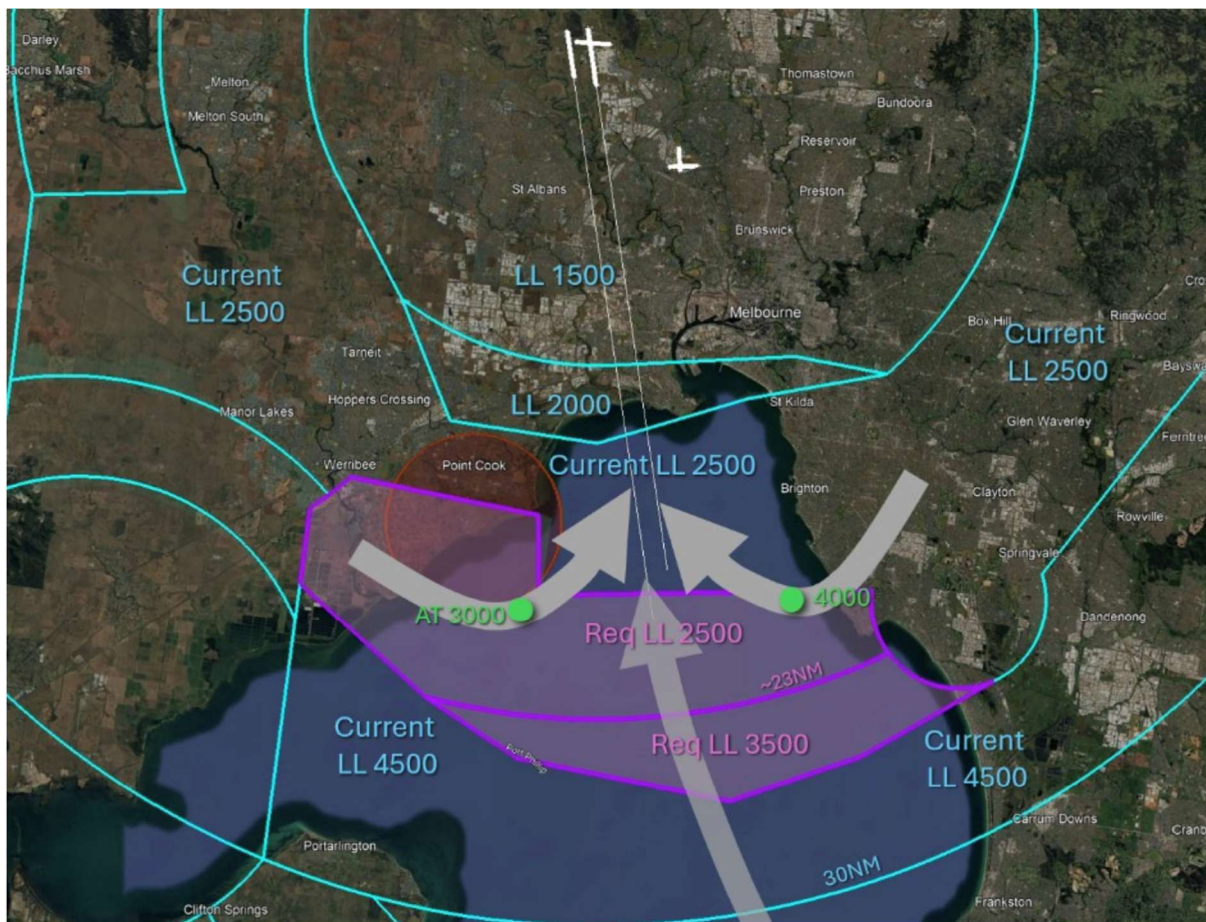
Figure 8: PHASE 1 - Initial proposed changes to control area steps to the south along with indicative aircraft altitudes for parallel arrivals.
