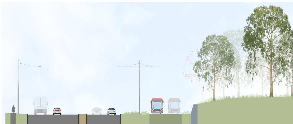
Figure 5-23 Indicative cross section of an inner running arrangement (in the Parliament House precinct on State Circle near Melbourne Avenue)
