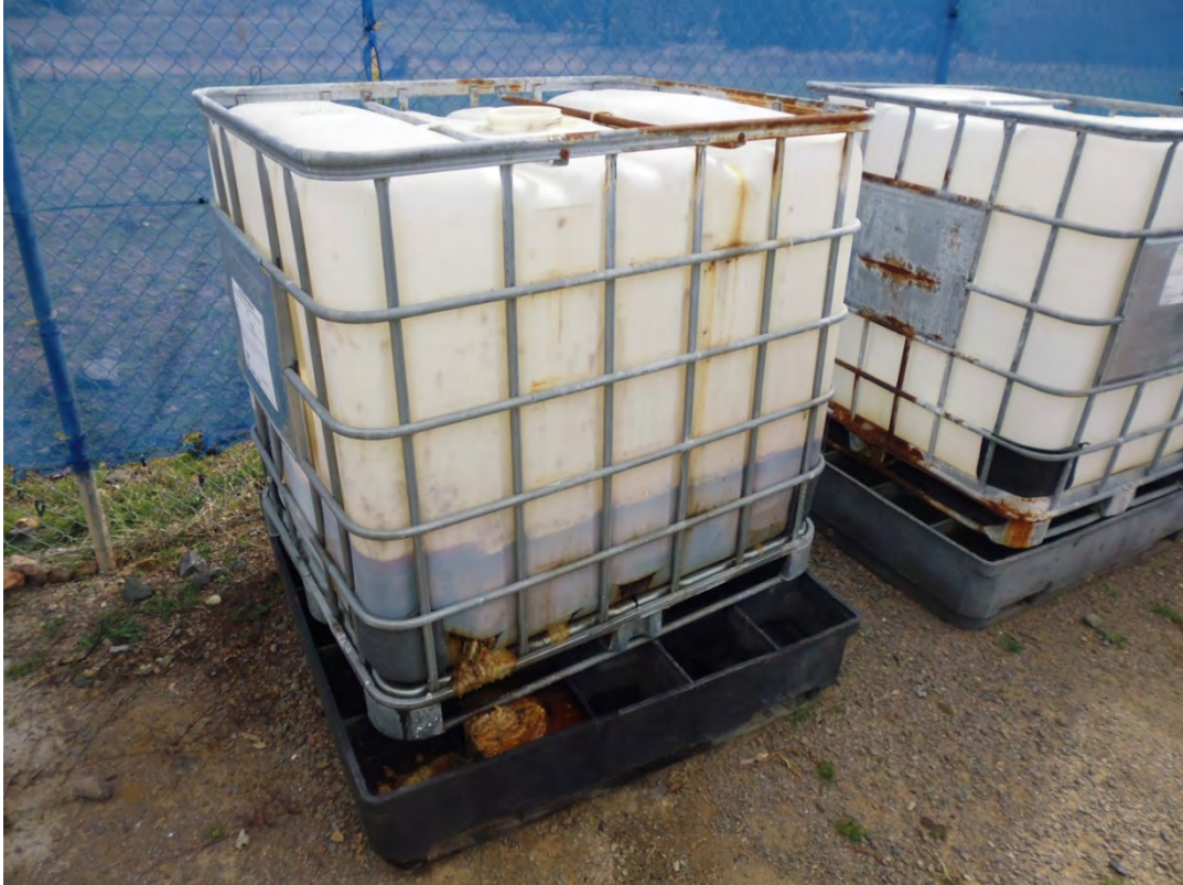
Photo 8 – Bunded pallets under IBCs stored in the open and partly filled with water.
