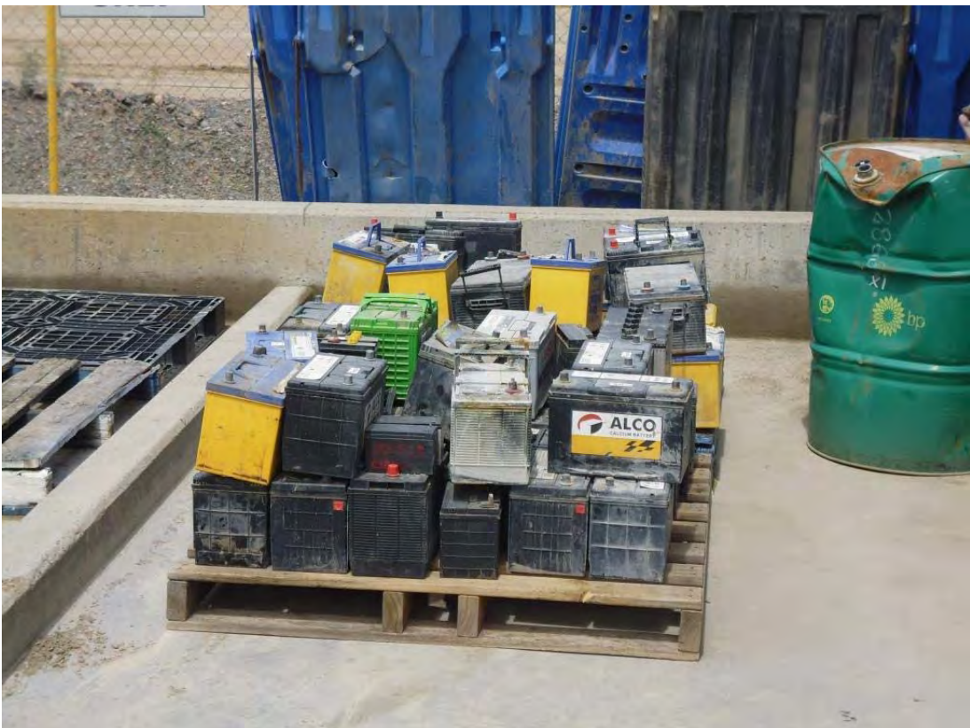
Photo 3 – Batteries stored in the open unbanded and not under cover at the Remondis waste compound.
