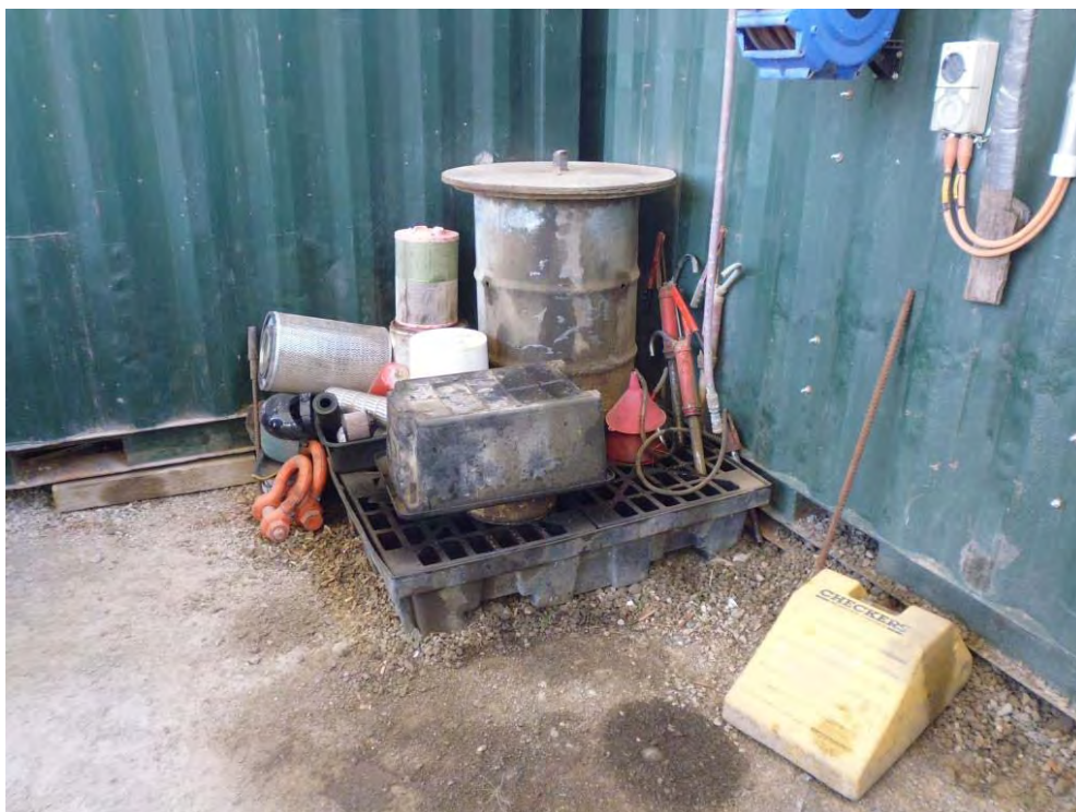
Photo 7 – Oil being drained into a bunded pallet in the open on bare soil, with the risk of the pallet filling with water during rainfall and overflowing onto the soil.
