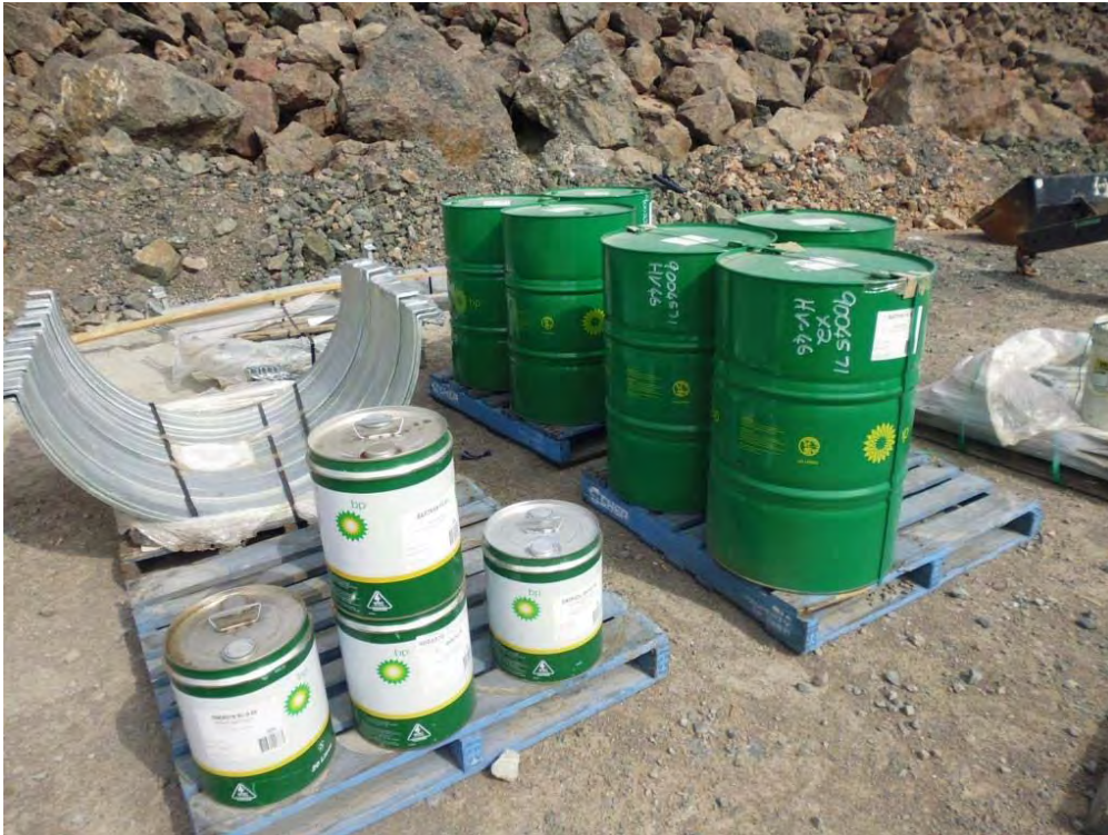
Photo 6 - Example of 200 litre and 20 litre drums stored unbunded in the open on bare soil at the PHE Electrical & Instrumentation Contracting compound.
