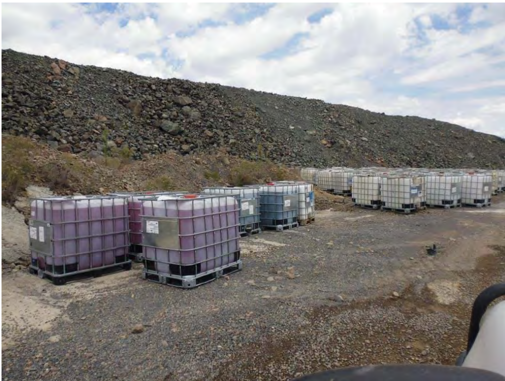
Photo 5 – Unbunded IBCs stored in the open on bare soil at the Boral Concrete Batching Plant.
