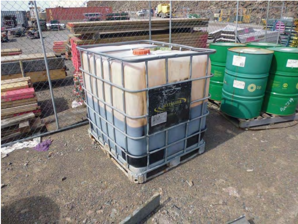
Photo 4 – Example of an IBC and 200 litre drums stored unbunded in the open on bare soil at the PHE Electrical & Instrumentation Contracting compound.
