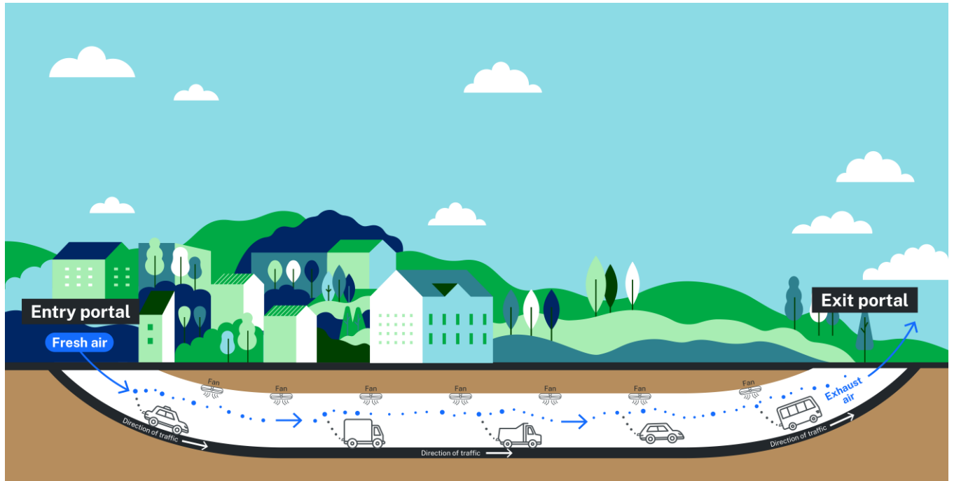
Figure 1: Tunnel ventilation through portals
