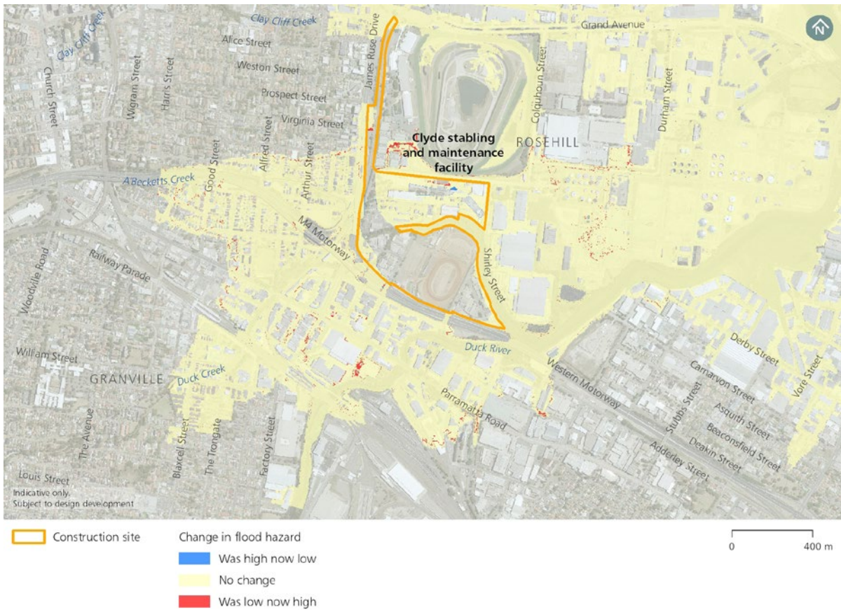
Figure 3-9: Potential change in flood hazard – probable maximum flood event as per Environmental Impact Statement compared to existing environment
