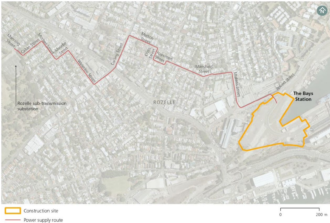
Figure 7-1: Exhibited power supply route for The Bays Station
