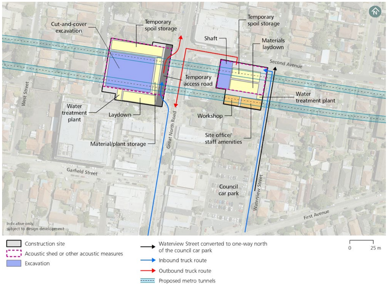
Figure 5-2: Amended road network modification at Five Dock Station construction site
