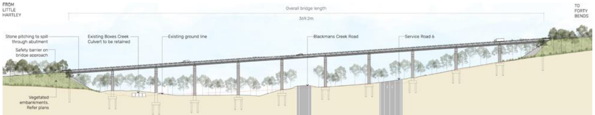
Figure 3-2 g Long section of the Great Western Highway twin bridges over Jenolan Caves Road
