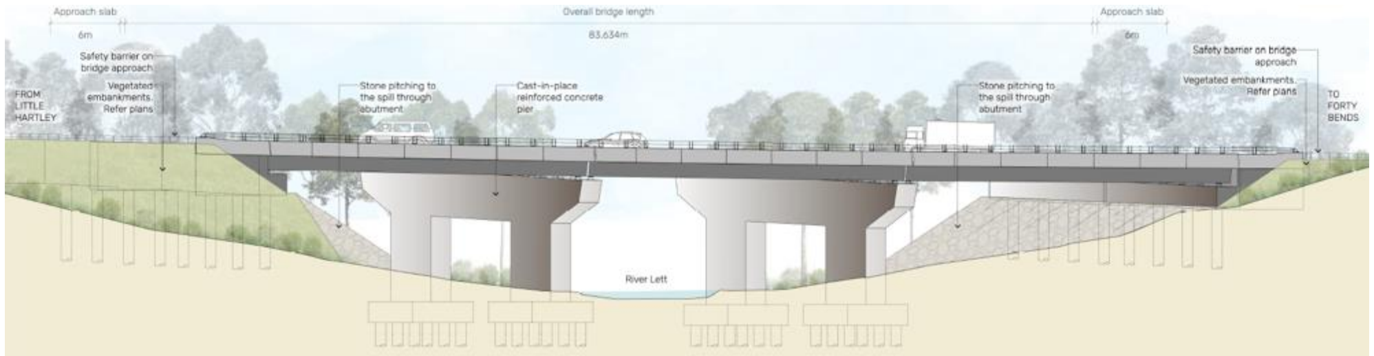
Figure 3-2 f Long section of the Great Western Highway twin bridges over River Lett
