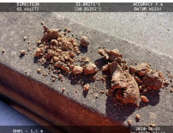
Photo 5: 28/10/2024: Photo of sandy silty clay fill at 1.5 mbgl of BH01
