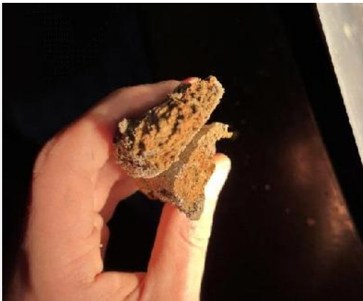
Photo 18: 20/11/2024: Photo of natural orange brown silty clay at 2.0 mBGL of BH10
