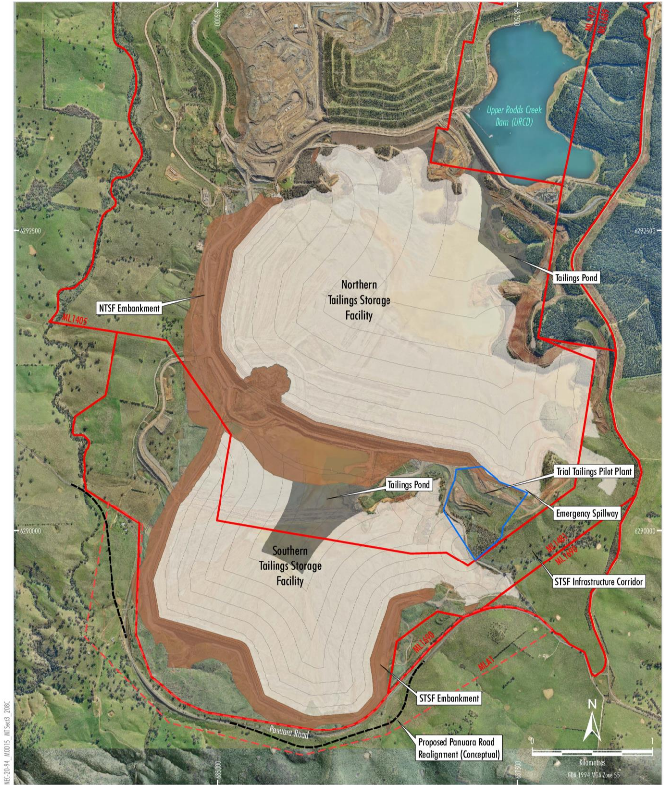
Figure 2: Extent of TSF Buttressing
