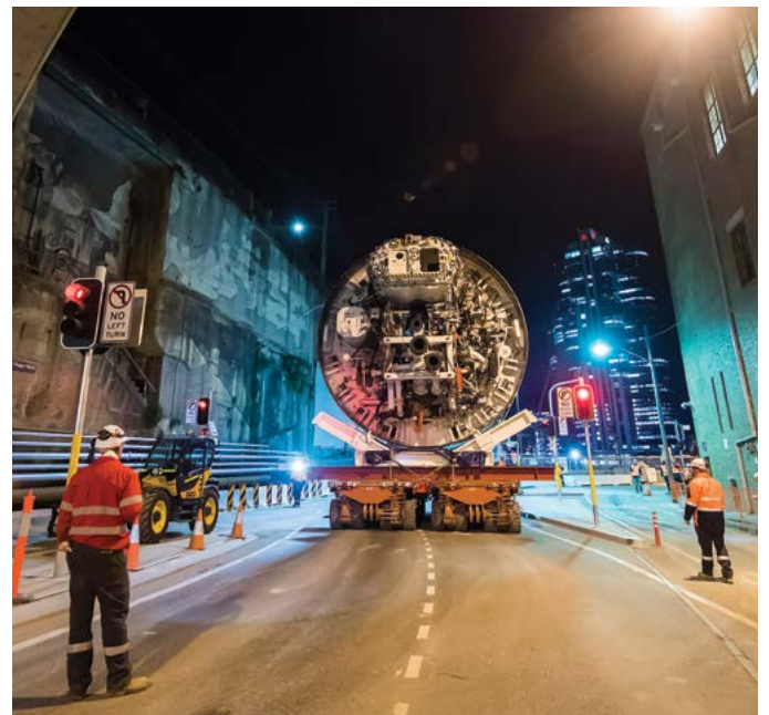
Tunnel boring machine used on the Sydney Metro project.
