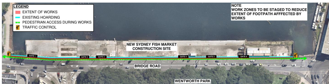
Figure 2: Pedestrian Access during works – Bridge Road
