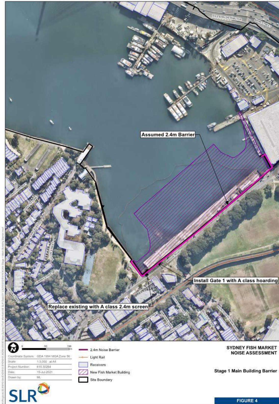
Figure 4 Stage 1 Main Building Hoarding Layout
