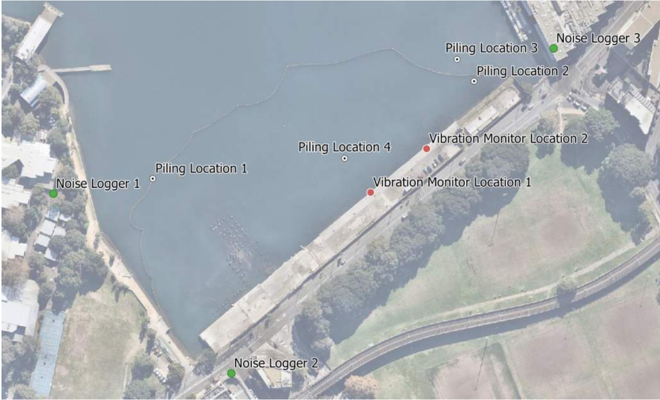
Figure C1 Vibration monitoring locations
