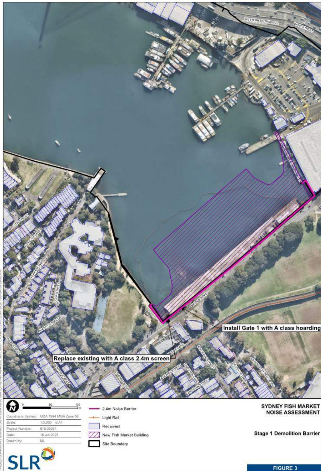
Figure 3 Stage 1 Demolition - 2.4m Hoarding Layout
