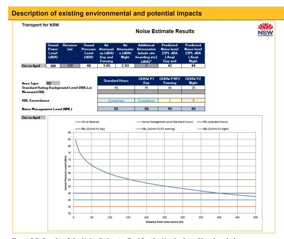
Figure 3.5: Results of the Noise Estimator Tool for the Hawkesbury River boreholes
