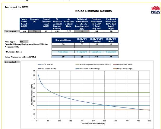
Figure 3.4: Results of the Noise Estimator Tool for the Brisbane Water borehole
