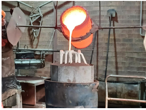
Bronze casting during fabrication, April 2024
